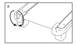
b. If the walking belt slips when walked on, first remove the key and UNPLUG THE POWER CORD.
